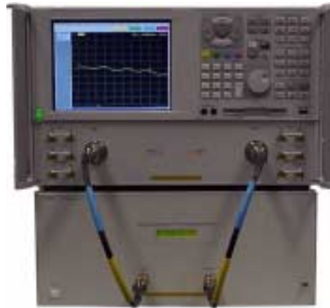
Figure 4 Connecting the Test Set to the Network Analyzer
